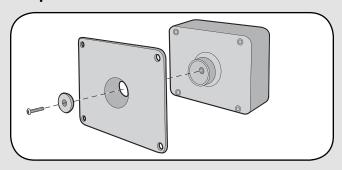
Attach PIR Motion Sensor box to mounting plate with large silver screw. Tighten screw until PIR Motion Sensor stays in place when repositioned.
